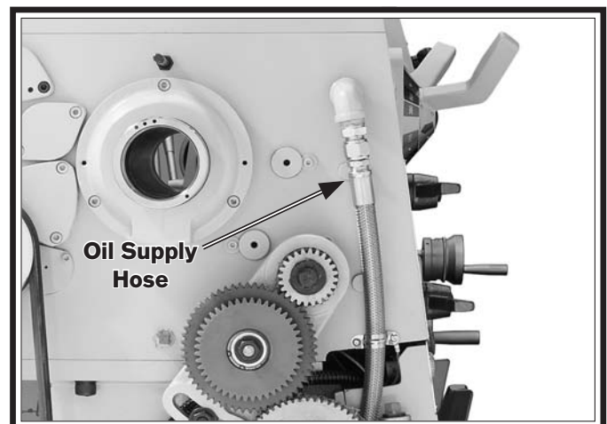
Figure 97. Headstock oil supply hose.
